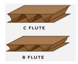
**\*B Flute Cardboard (Type B) -** cardboard has excellent crush and puncture resistance and is a great printing surface. This cardboard is commonly used forinner packaging components such as pads and partitions
