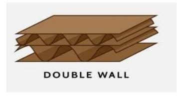
\*Double wall board has two layers of corrugated fluting and three liners, makingit extremely durable.
