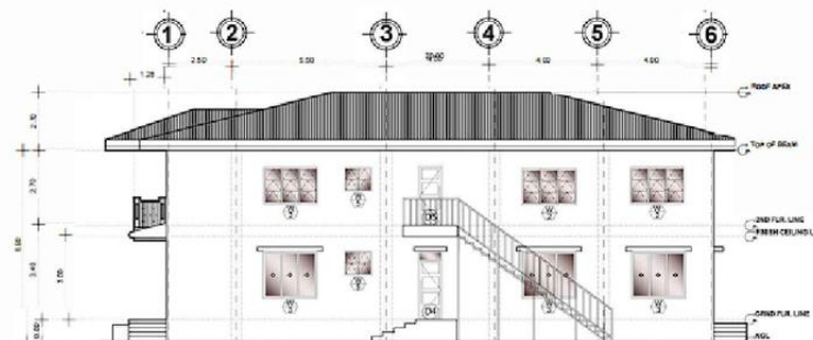
RIGHT SIDE ELEVATION SCALE: 1:100 MTS
